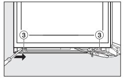
Slide the soft-close mechanism back into the door as far as it will go towards the appliance using a flat-headed screwdriver.
